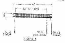
Detail drawing of fabricated coil L1. Make no substitutions and follow plan carefully.
