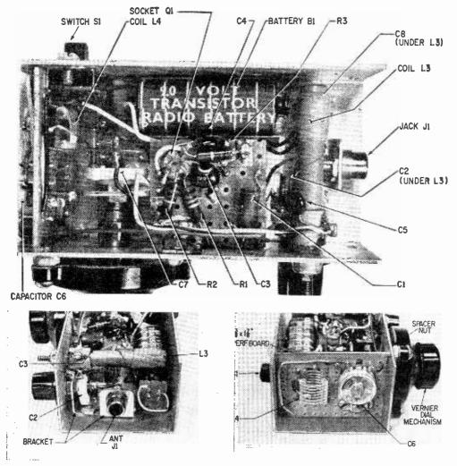
Various views of chassis show the mounting of perf boards, and the location of components.
