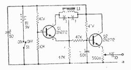
The oscillator circuit shown in the diagram employs two transistors. Its frequency depends upon the inductance value of audio frequency choke L1. It can be the primary winding of an output transformer when the secondary winding is not used.
