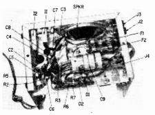
formed by C9A, C9B, and resistor R6. The B+ and 6.3 vac power supply voltages are connected through fuses F1 and F2 to the external pin jacks allowing the amplifier to be used as a power supply for low power appli-
