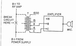
can be varied by trying various amplifier output and transformer connections such as 8-ohm or 16-ohm amplifier output to 4, 8 or 15-ohm transformer lead. Set the amplifier tone controls to reduce high frequency response so you won't cause excessively wide side bands to be produced.
