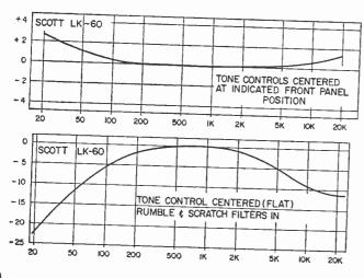
Fig. 1. Frequency response curve plotted with tone controls centered shows response boosted less than 3 db at 20 cycles. Adjustment of controls gives flat response within 1 db.
