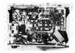
The HB-600 rig sports separate PC's for receiver, transmitter and audio—all solid-state.
