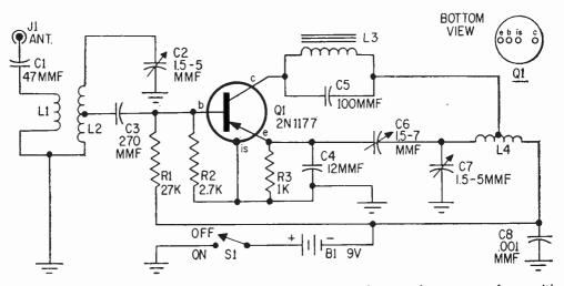
Schematic diagram of the Aero-Bander: notice the apparent absence of any output from unit!
