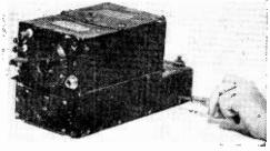
Area behind power plug, left, is tightly packed. Above, BFO oscillator is adjusted.
