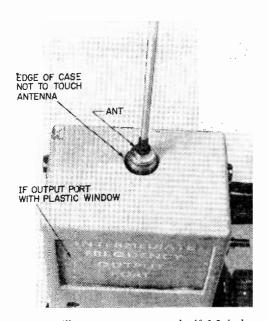
Close-up views of front panel and top of the chassis show details of construction. Notching of chassis for L3 and tuning dial is shown above; antenna mounting details and
