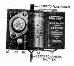
The handful of electronic parts that make up the Transiflash fit neatly on a 1% x 2-inch phenolic board as shown above. Dry cell battery (below) juts past board and is held in place by its leads. Entire unit can be potted with only the battery outside.
