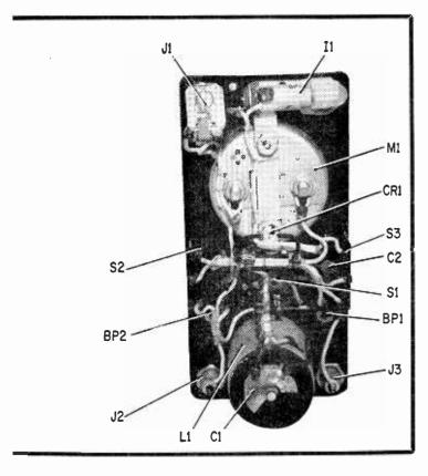
All components mount behind front panel. At top is bulb, with tuning capacitor C1 at the bottom. Be sure to use a plastic case, not metal, to assure adequate RF pickup.
