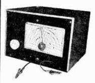
A piece of scrap aluminum and a 3x5 filing card are the no-cost materials required for this calibrating dial
