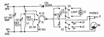
Schematic. Tuned circuit at left selects signal; CR1 converts it to DC.
