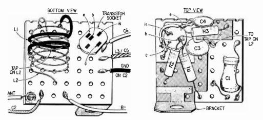
Top and bottom of larger of the two perf boards are shown here for construction details.
