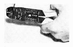
Electrical crimp is made on 12-10 AWG using marked notch and closing tool completely.
