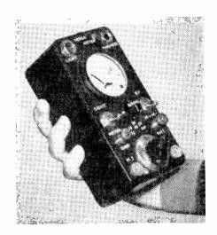
Build this little gem for your ham shack. It's a wavemeter, field-strength indicator, phone monitor and milliammeter all rolled in one. It'll help keep signals clean and legal.
