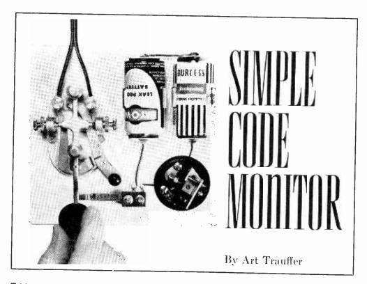
■ Most of us send better code when we can hear what we're sending. This code monitor, which is entirely independent of your receiver or transmitter and has no electrical connections to any of your equipment, is quickly rigged up using only three main components: first, a pair of prongs or reeds from an old phone jack, switch, or relay; secondly, a 3-volt supply (two D batteries); and, finally, a buzzer.
